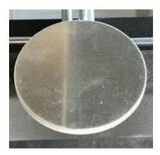
The entire field of glass will be protected by acrylic-coated, polycarbonate (Extended Life Lexan - XL10<sup>TM</sup>). The acrylic coating is harder, providing more resistance to scratching, and it protects the polycarbonate from ultraviolet (sun) light to reduce yellowing. The polycarbonate is virtually shatter proof providing a greater level of security for the stained-glass windows.
